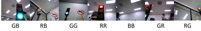
Figure 12: Examples of detection results ('G' - Green, 'R' - Red, 'B' - Blank). The first letter of the image label (e.g., 'R' of 'RB') represents the ground truth of the image, while the second letter represents the detection result.
